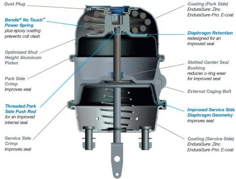
Not all spring brakes are created equal. Many competitive suppliers have made the choice to introduce low-cost products by compromising on design and components that stop short on quality.
